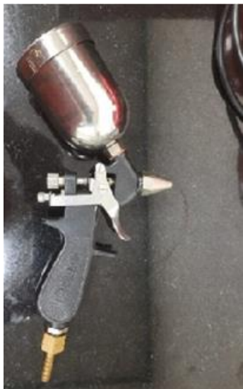
Fig. 3 Photograph of powder spraying arrangement
