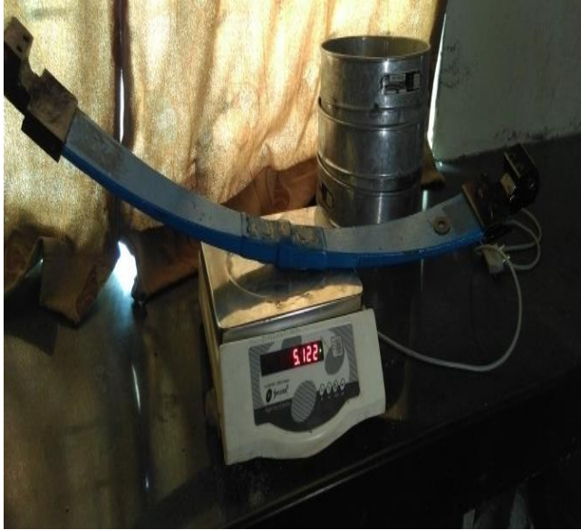
Fig. 1 The mass of the composite mono leaf spring with eye
