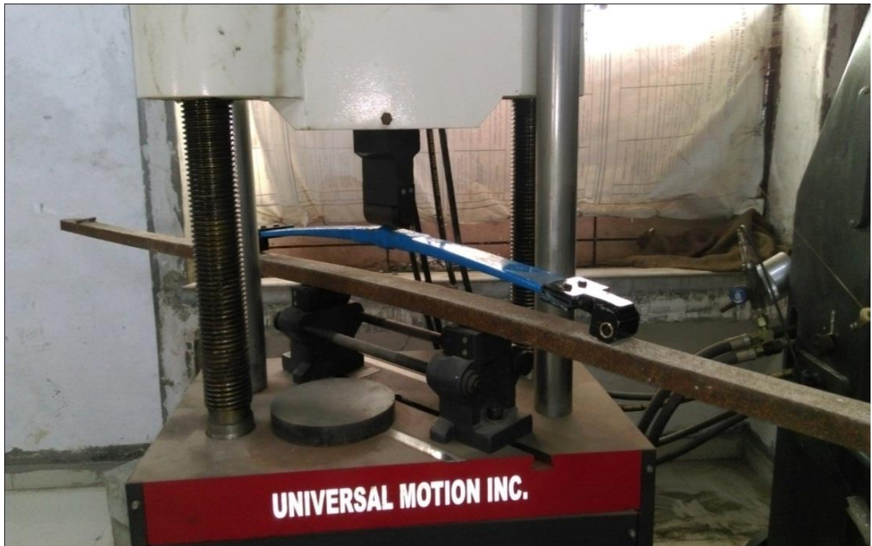
Fig. 4 Static stiffness test on UTM
