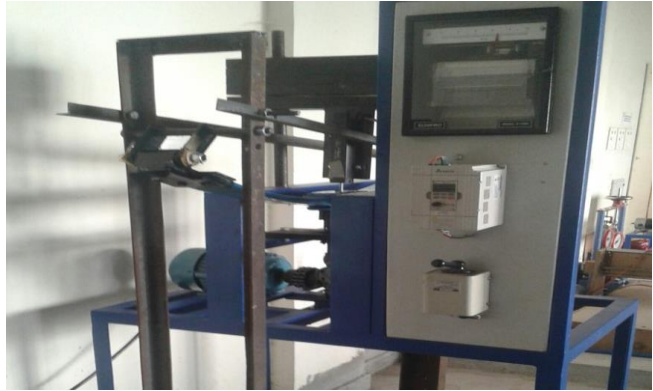
Fig. 7 Transmissibility evaluation test setup front view
