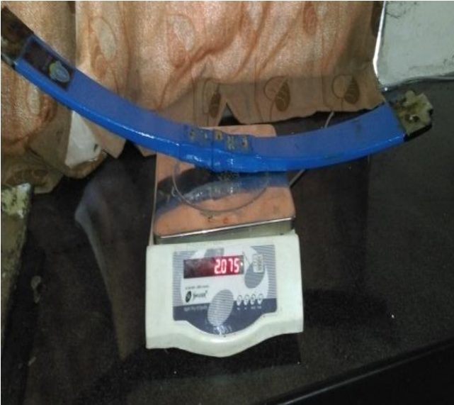
Fig. 2 The mass of the GFRP composite mono leaf spring without eye
