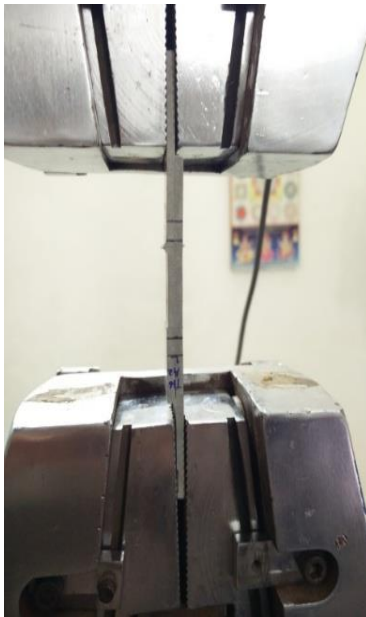
Fig. 13 Tensile-shear testing of specimen on universal testing machine M-100, FSA
