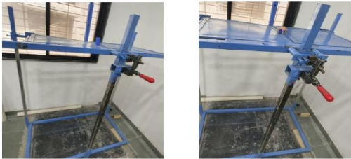
Fig. 7 Drop and impact test set up of lithium ion battery
