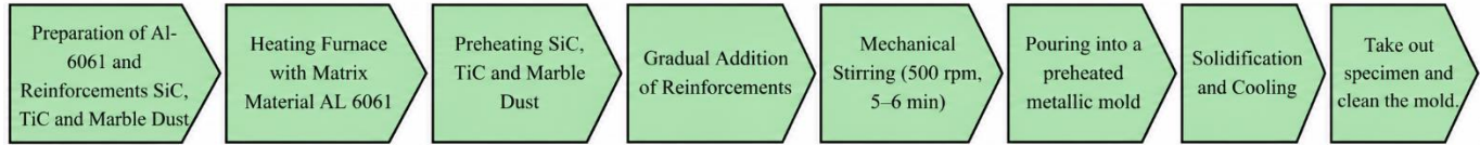
Fig. 1 Flow chart of stir casting process and reinforcement addition sequence for the fabrication of AA6061 hybrid composites
