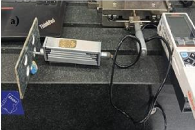
Fig. 5 (a) Surface roughness experimental setup, (b) Test samples.
