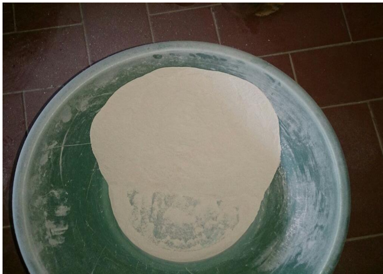
Fig. 2 Sieved eggshell particles of 150 micron size
