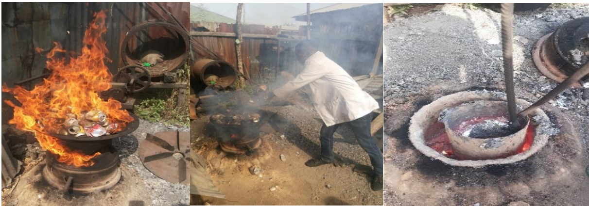
Fig. 4 Melting compressed cans in a furnace
