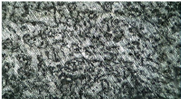
Fig. 14.2. Micrograph of 2 wt% Sample (X100)
