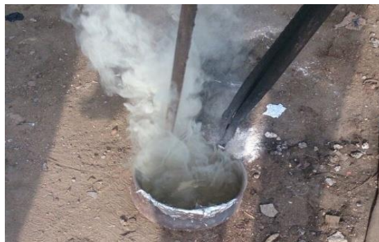
Fig. 5 Mixing and stirring of ES particles with the molten metal in the ladle
