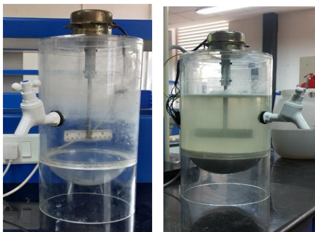
Fig. 2 Blade agitator device utilized for struvite crystallization development
