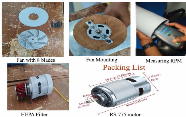
Fig. 11 Components and Assembly of the Two-Wheeler-Mounted Dust Collection Sampler
