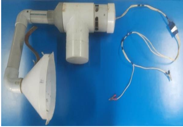
Fig. 17 Fugitive vehicular mobile dust collector prototype (actual)
