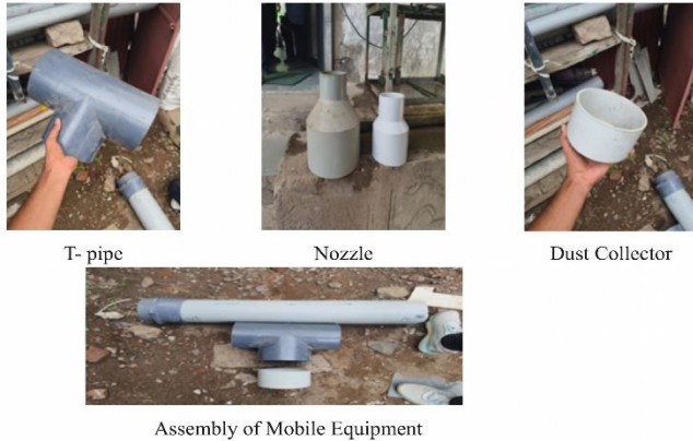
Fig. 10 Material and part of the mobile dust sampler
