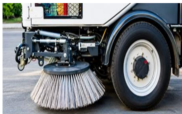
Fig. 6 Spinning brush-type road dust collector [28]
