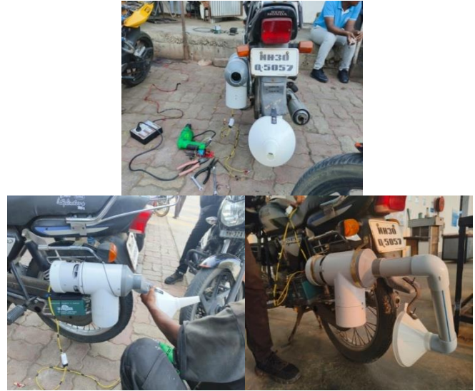
Fig. 12 Installation of a mobile dust collection sampler on two two-wheeler vehicles
