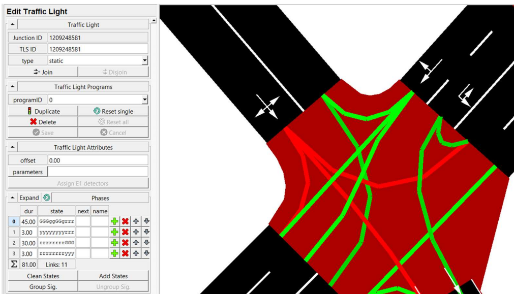
Fig. 6 Traffic lights phase durations, state strings, and total cycle length settings in NETEDIT.
