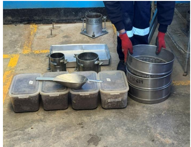
Fig. 9 Modified Proctor compaction and equipment during execution
