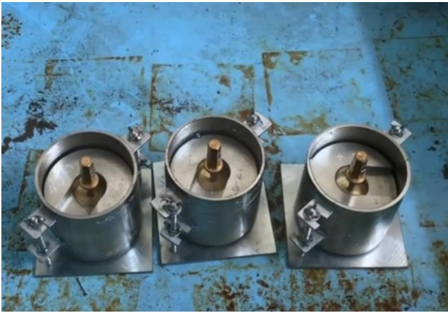
Fig. 10 Preparation of samples for CBR testing
