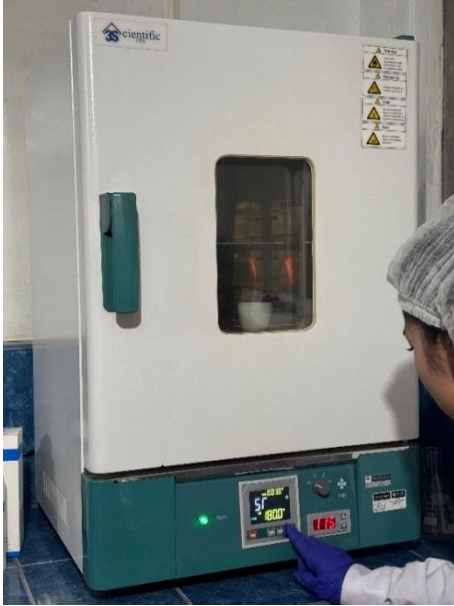
Fig. 8 Water reduction in soil samples by heat
