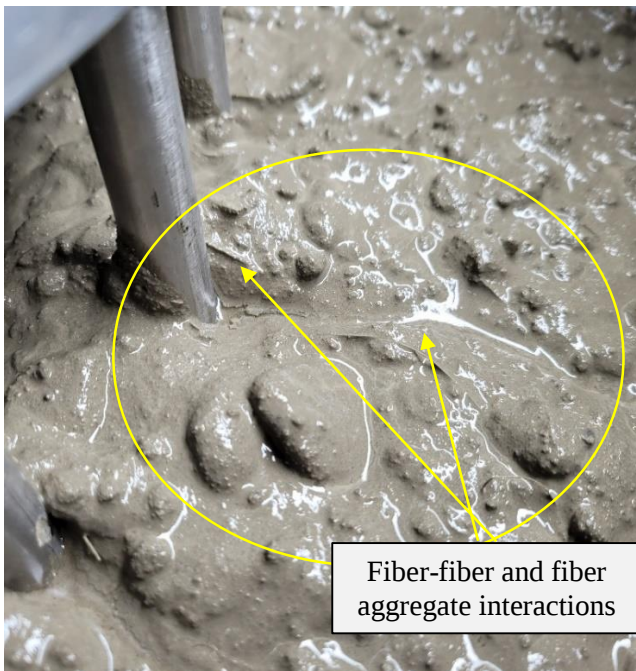
Fig. 19 Fiber-fiber and fiber-aggregate interactions
