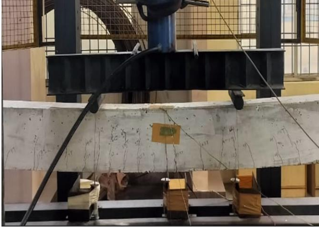
Fig. 8 (b) Formation of Crack pattern of GP50M4 mix GRC beam
