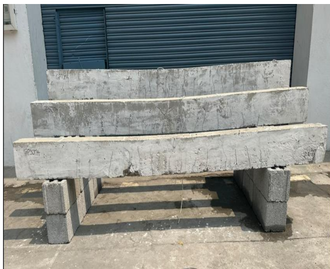
Fig. 11 Tested GPC beams of GP30M4, GP50M4 and GP70M4 mixes
