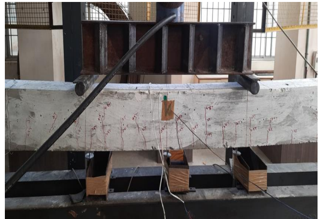
Fig. 8 (a) Formation of crack pattern of GP30M4 mix GRC beam
