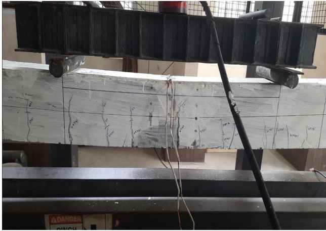
Fig. 8 (c) Formation of Crack pattern of GP70M4 mix GRC beam
