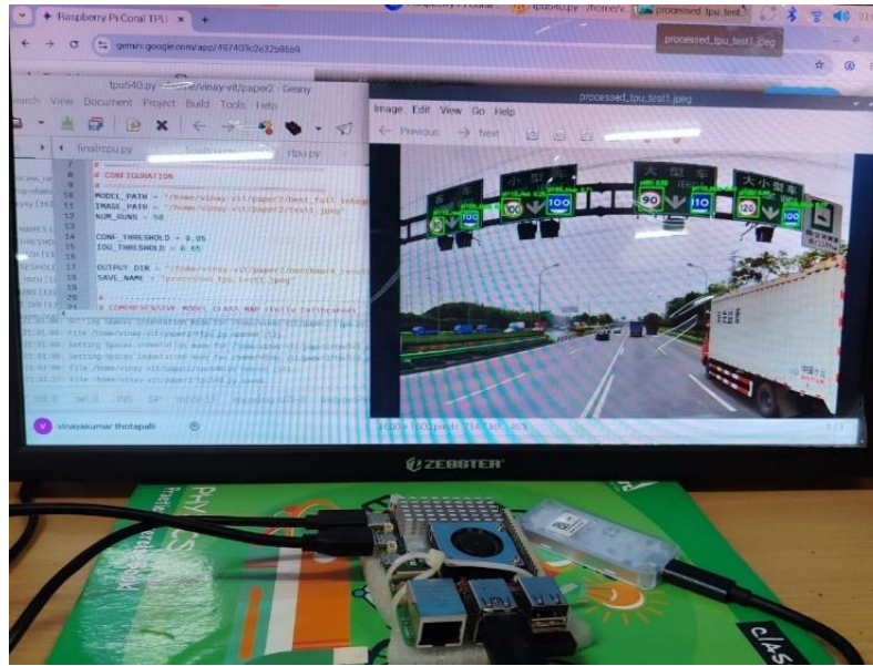
Fig. 2 Physical test setup: RPi 5 with the Coral USB Edge TPU running live inference
