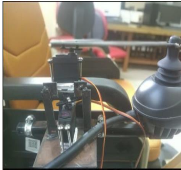
Fig. 13 Designed a control interface to control the joystick of the Electric wheelchair
