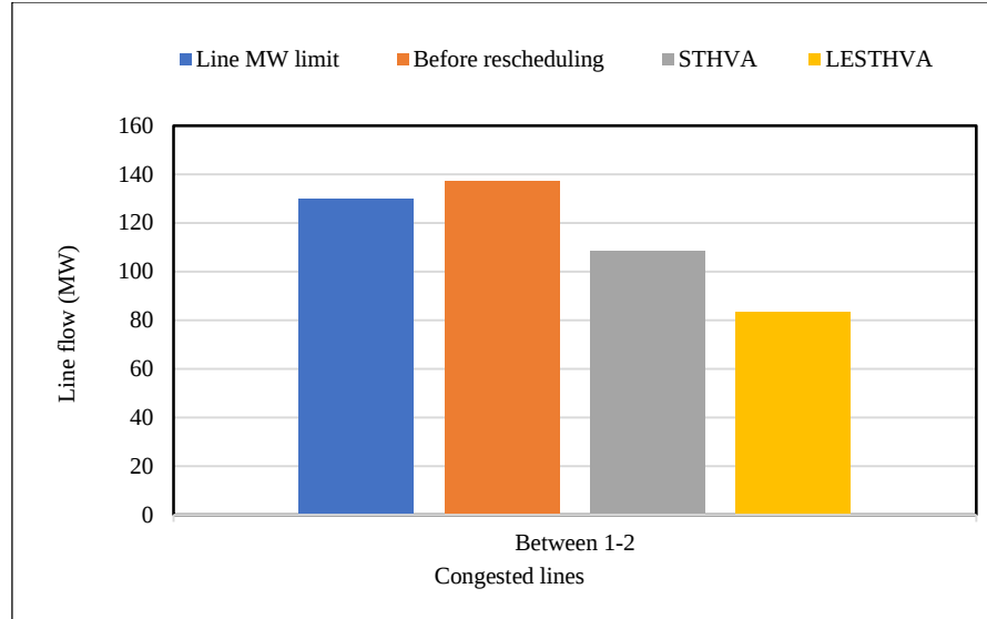
Fig. 5 Power flow in congested lines-comparison in case 3
