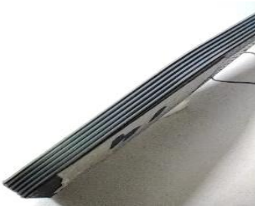
Fig. 2 Alternating-layer deposition in ABS-PC printed specimen
