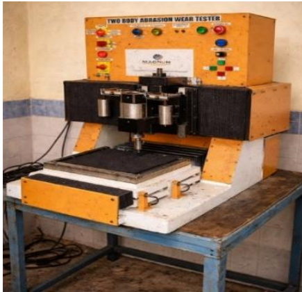
Fig. 5 Two-Body Abrasive Wear Test setup
