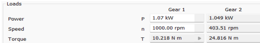
Fig. 2 Kinematic verification of the train (DIN 3990) and pass parameters for the initial case (P, n, T).
