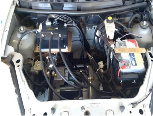
Fig. 3 Electric motor and powertrain components of the Innowattis project
