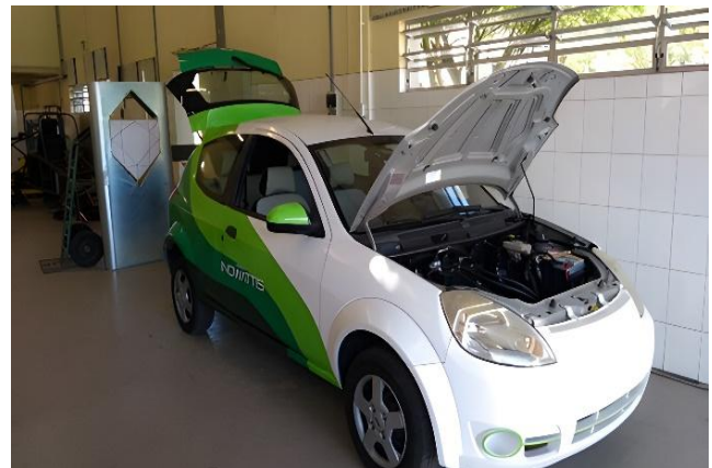
Fig. 2 Converted Ford Ka (Innowattis project) developed at SATC
