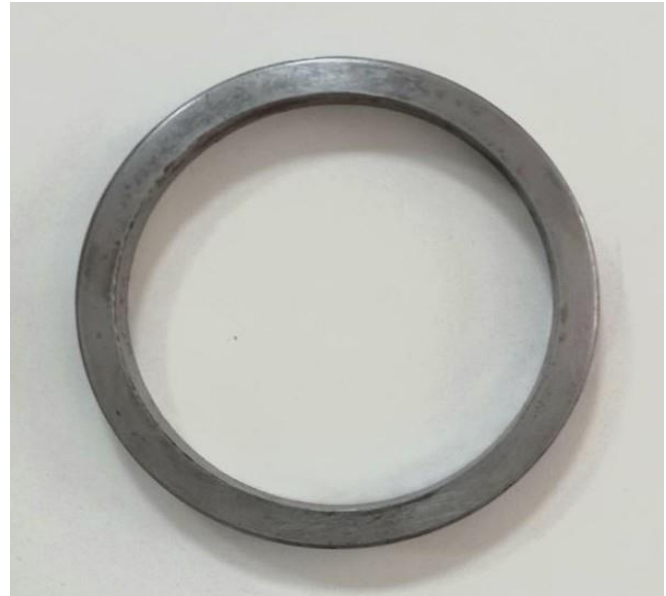
Fig. 2 Toroid shaped specimen photograph after hard sintering
