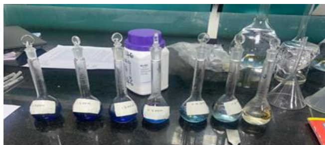
Fig. 14 Decreasing color intensity leads to a lower concentration of phospholipids
