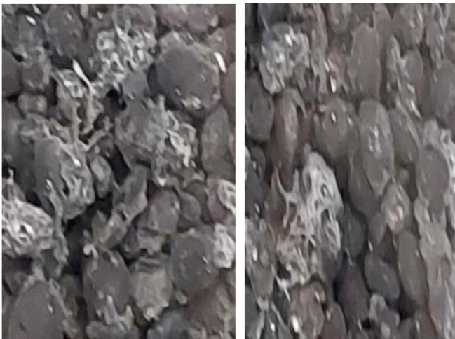
Fig. 10 Gelatinous material formation on the granular biomass due to 30 ppm Solutrix100 application
