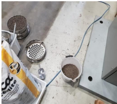
Fig 1: LECA Laterlite expanded clay in a granular form before sieving
