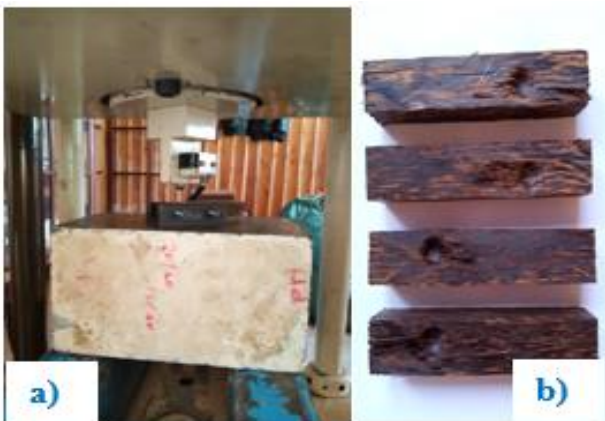
Fig. 6: Janka hardness test: a) Specimen testing; b) Specimen's failure
