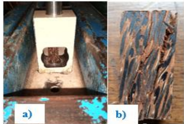
Fig. 4: Compression parallel to grain test: a) Specimen in compression; b) Specimen's failure
