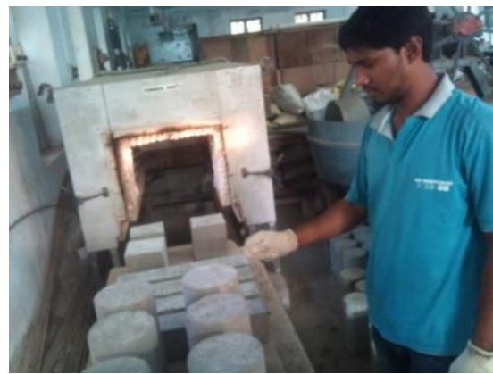
Fig. 2 Bogie furnace with specimens
