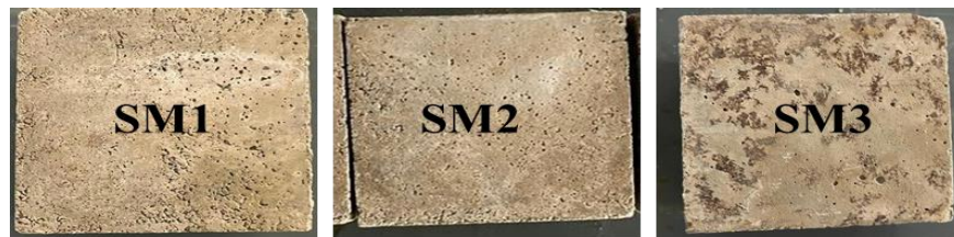
Fig. 5 Visual deterioration of samples SM1, SM2 and SM3 after exposure to sulphate attack for 90 days at 5% sulphate concentration
