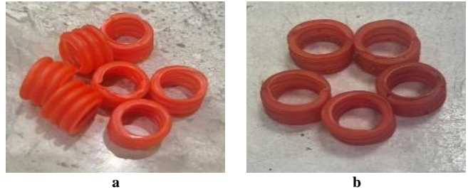
Fig. 7 Pieces of spiral electric hose a) Before using it b) After the operation period.
