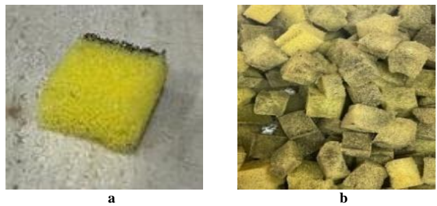
Fig. 9 Artificial Sponge a) Before using it b) After the operation period
