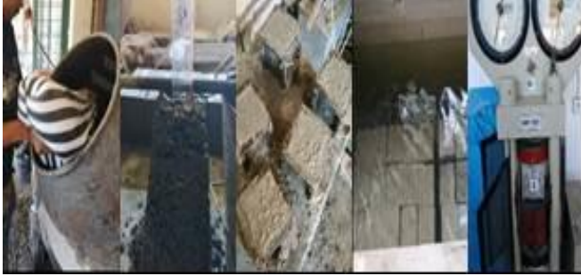
Fig. 3 Mixing, casting, curing and testing
