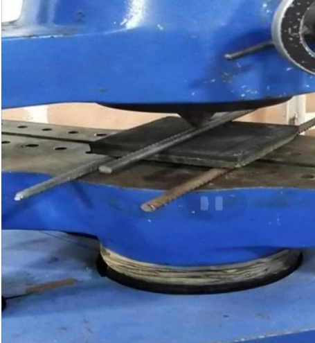
Fig. 7 Testing of tiles for transverse strength in UTM
