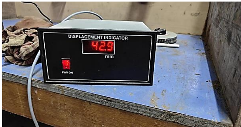
Fig. 4 Displacement indicator for deflection measurement
