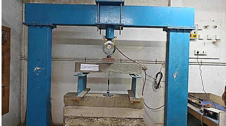
Fig. 3 Experimental setup for the deflection test
