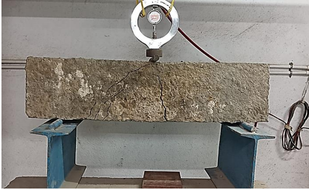
Fig. 5 Cracks in beams
