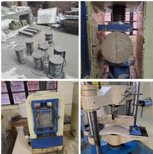
Fig. 1 Casting and testing of concrete specimens
