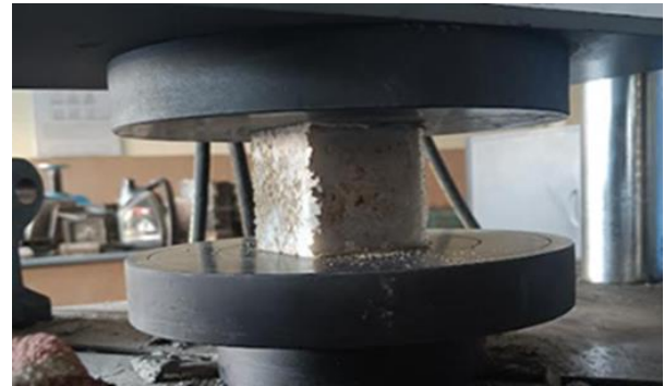
Fig. 6 Plastic-sand block at the point of cracking
