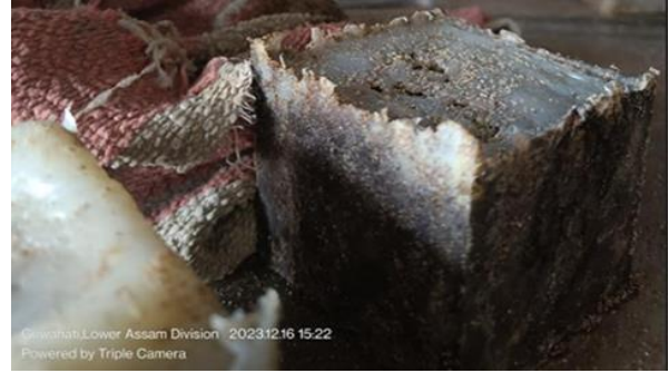
Fig. 5 Plastic-sand block prior to testing
