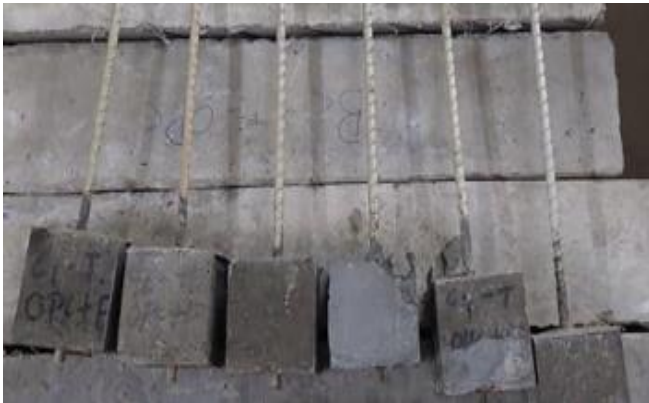
Fig. 4 Plain concrete specimens with GFRP rebar exposed to chlorine
