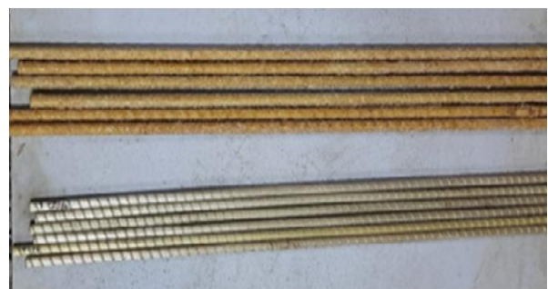
Fig. 1 GFRP rebars (Twisted and sand-coated)
