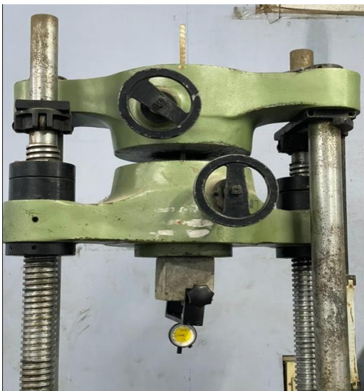
Fig. 3 Pullout test setup
