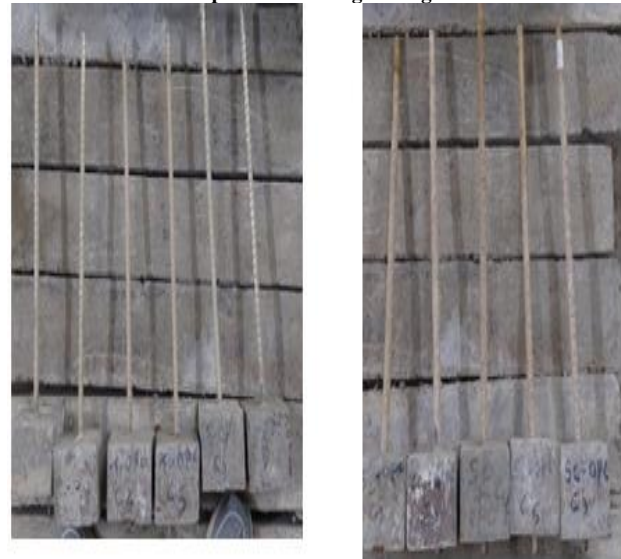
Specimens after 180 Days of exposure to chlorine GFRP rebar twisted, GFRP rebars and coated Fig. 2 Pullout specimen details
