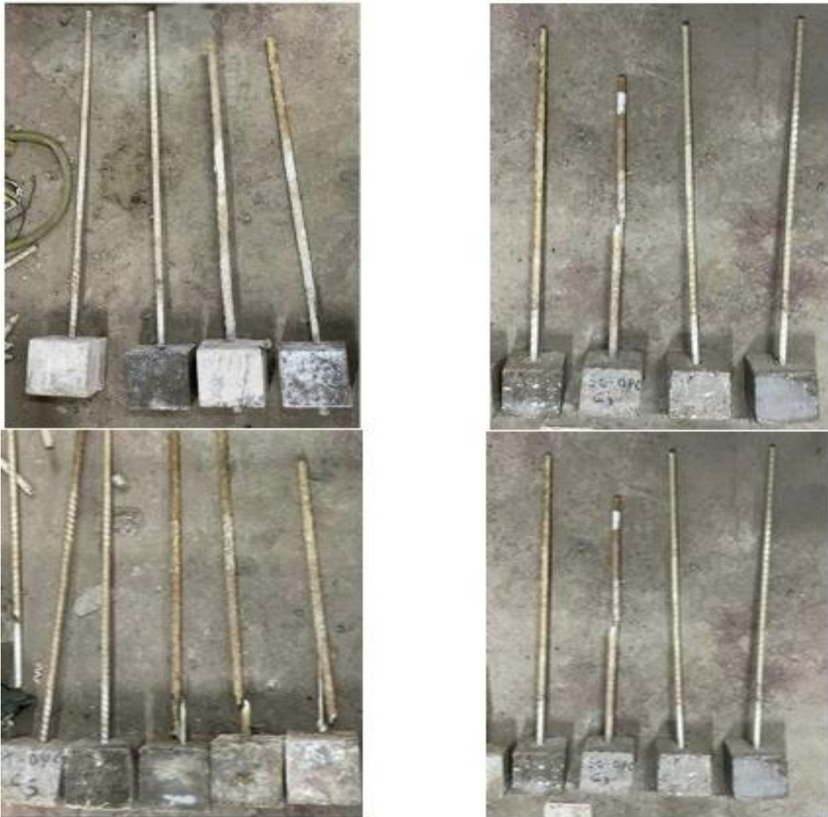
Fig. 12 Failures modes of GFRP (Sand-coated/Twisted) rebars@ direct pull out test after 180 days of exposure under marine/conventional exposure conditions
