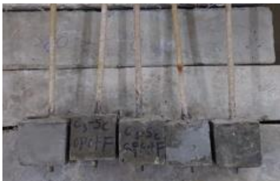
Fig. 5 FRC specimens with GFRP rebar exposed to chlorine
