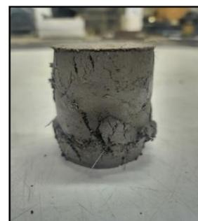
Fig. 14 UCS failure pattern of soil-areca fiber mix at 28 days curing period
