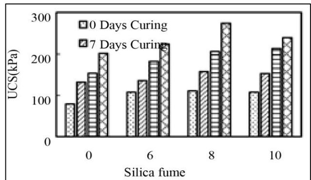
Fig. 9 Variation of UCS of soil and silica fume with respect to change in curing days and percentage of SF.
