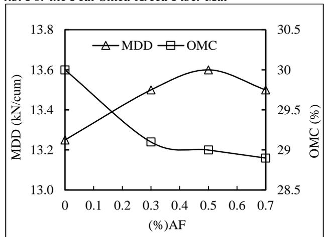
**Fig. 8 Variation of MDD and OMC of Soil+6%SF+(%)Areca fiber mix**
