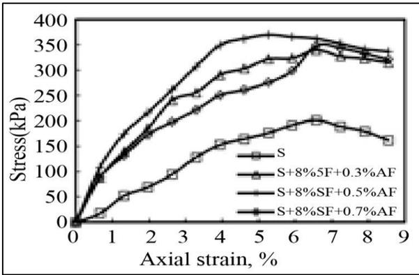
Fig. 19 Stress-strain curve for different mixes of 8% SF and %AF with soil at 28 days curing period
