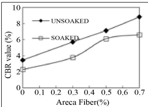
Fig. 23 Variation of unsoaked and soaked CBR of soil-areca fiber mixes
