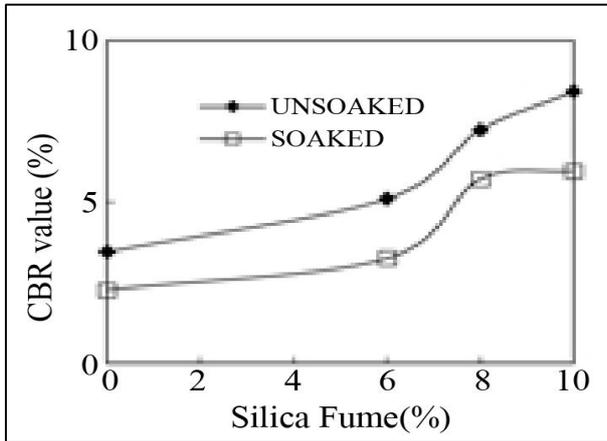
Fig. 22 Variation of unsoaked and soaked CBR of soil-silica fume mixes
