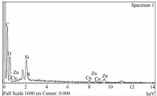
Fig. 32 EDX result of areca fiber
