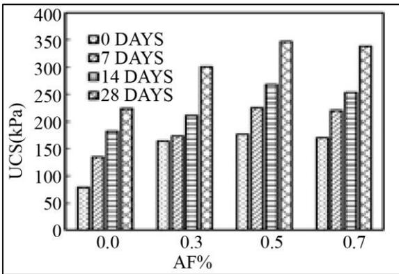
Fig. 15 Variation of UCS of soil and 6% silica fume with respect to change in curing days and percentage of areca fiber
