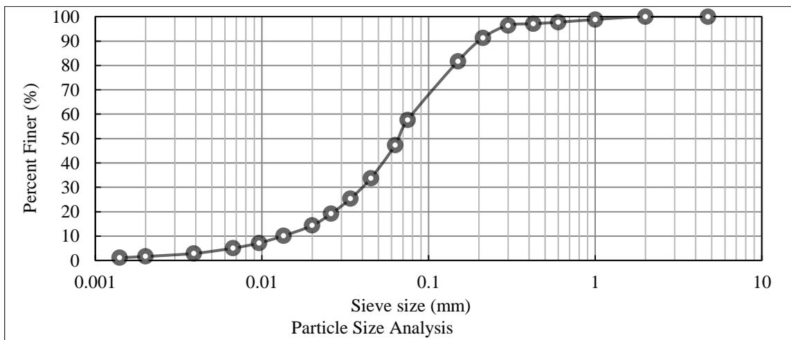
**Fig. 1 Particle size distribution curve of peat soil**
