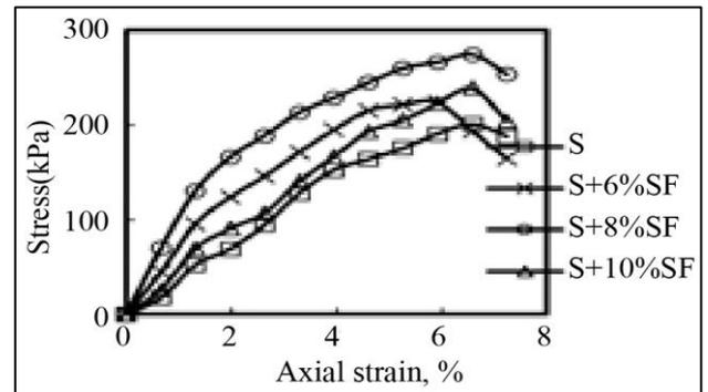
Fig. 10 Stress-strain curve for different mixes of Silica fume with soil at 28 days curing period
