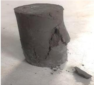
Fig. 11 UCS failure pattern of soil-silica fume mix at 28 days curing period
