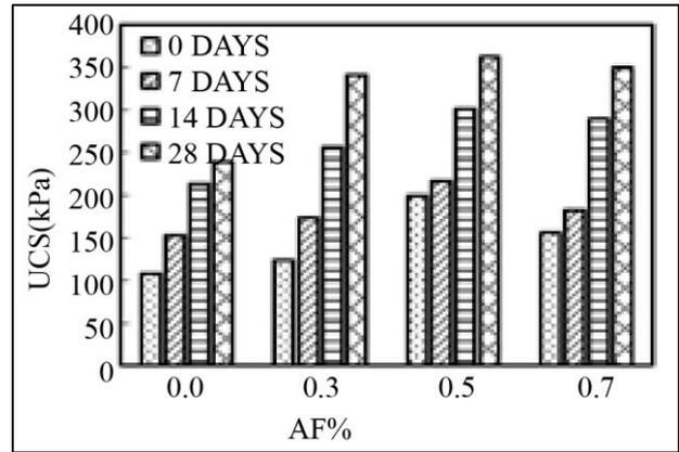
Fig. 17 Variation of UCS of soil and 10% silica fume concerning change in curing days and percentage of areca fiber
