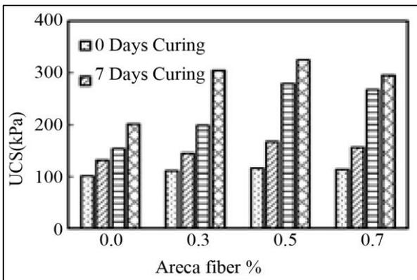
Fig. 12 Variation of UCS of soil and areca fiber with respect to change in curing days and percentage of AF
