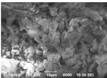
Fig. 29 SEM images of silica fume
