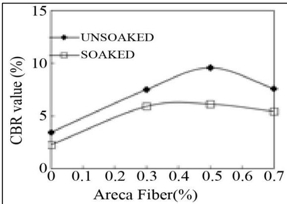
Fig. 25 Variation of unsoaked and soaked CBR for different mixes of 8% SF with soil
