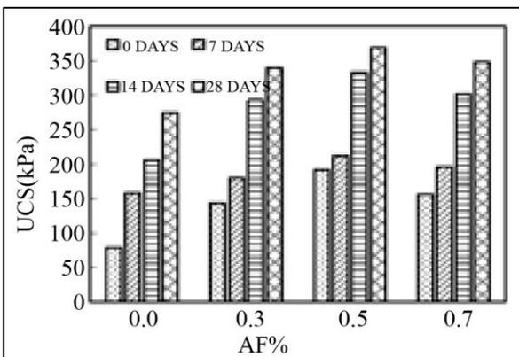
Fig. 16 Variation of UCS of soil and 8% silica fume with respect to change in curing days and percentage of areca fiber
