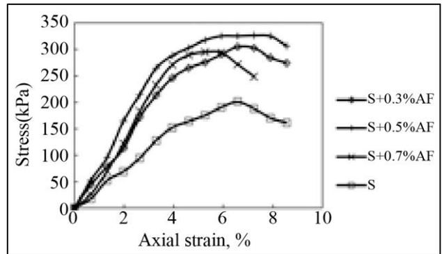
Fig. 13 Stress-strain curve for different mixes of areca fiber with soil at 28 days curing period
