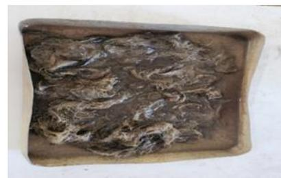
**Fig. 5 Areca coir immersed in water with linseed oil**
