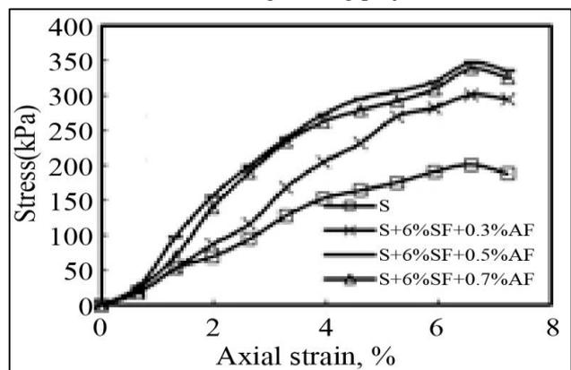
Fig. 18 Stress-strain curve for different mixes of 6% SF and %AF with soil at 28 days curing period
