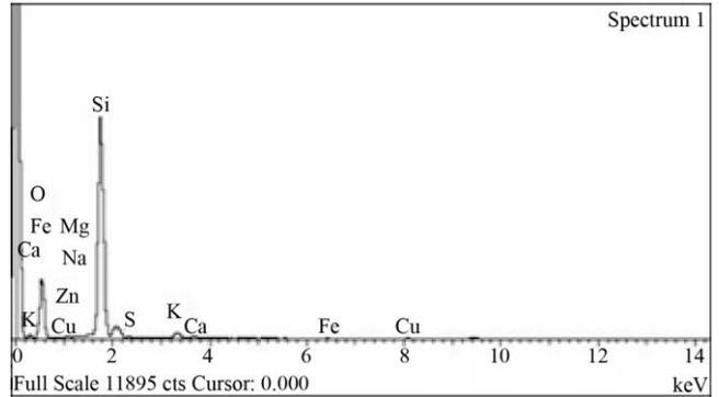
Fig. 30 EDX result of silica fume
