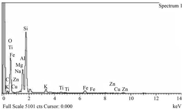
Fig. 28 EDX result of untreated peat soil
