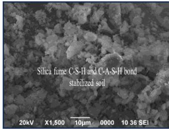
**Fig. 33 SEM images of soil-silica fume mix**
