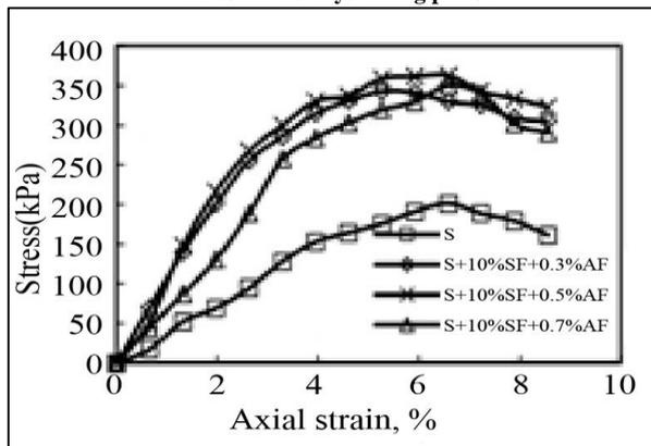
Fig. 20 Stress-strain curve for different mixes of 10% SF with %AF with soil at 28 days curing period
