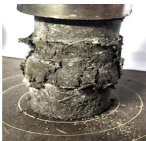
Fig. 21 UCS Samples of soil-SF-AF mix and failure pattern at 28 days curing period
