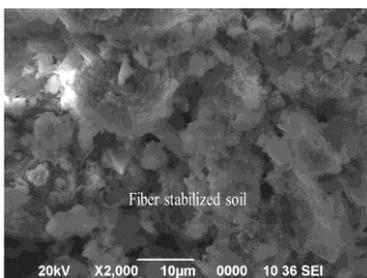
**Fig. 34 SEM images of soil-areca fiber mix**
