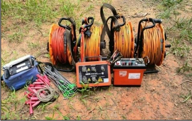
Fig. 9 Resistivity survey equipment – ABEM SAS4000
