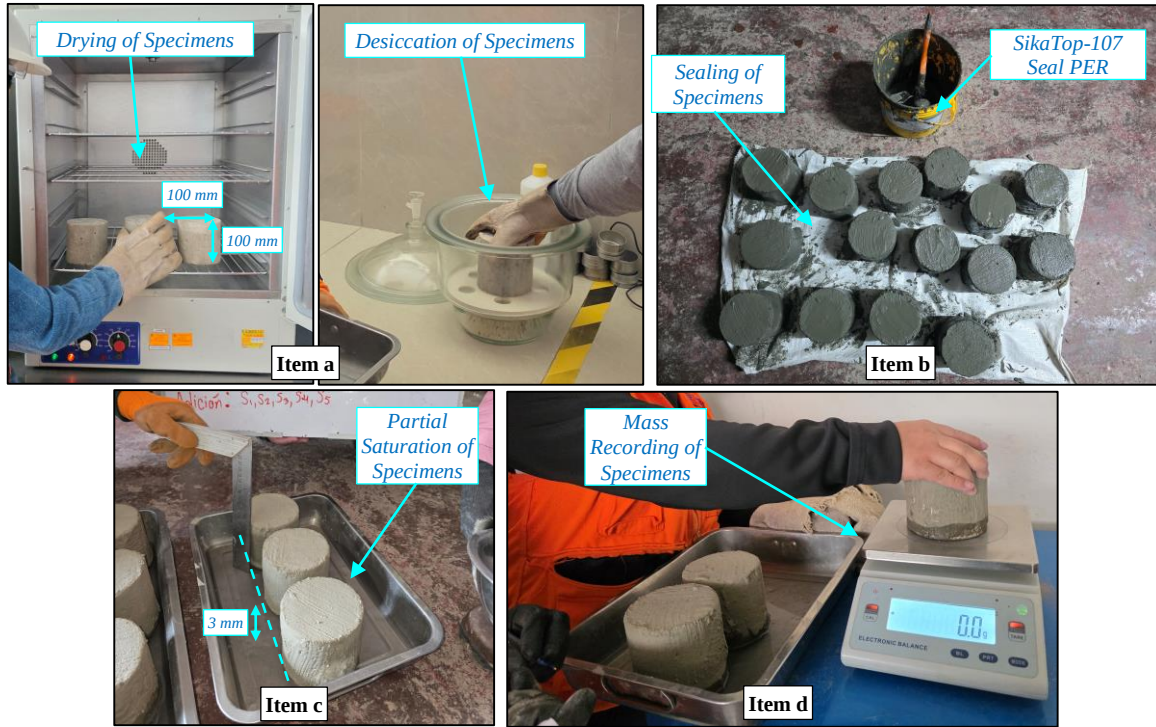
Fig. 15 Sorptivity test procedure
