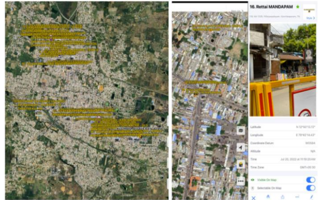
Fig. 11 Thirty-four Mandapams georeferenced using a walkover survey using the Map-plus application. Source: Authors
