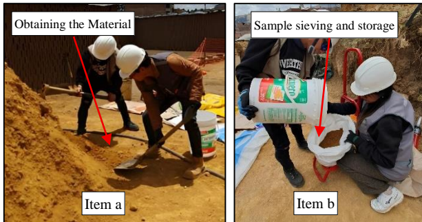
Fig. 1 Soil selection procedure for adobe
