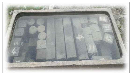
Fig. 4 Water curing of test specimens up to 28 days
