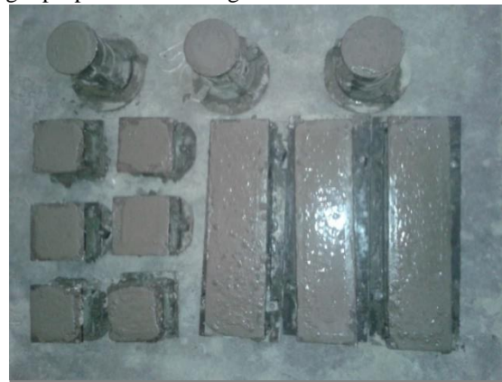
Fig. 3 Casting of concrete specimens for mechanical testing
