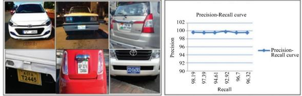
Fig. 7 A Precision-Recall Curve for Images of Multiple-Line Licence Plates
