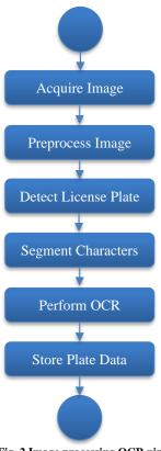
Fig. 2 Image processing OCR pipeline
