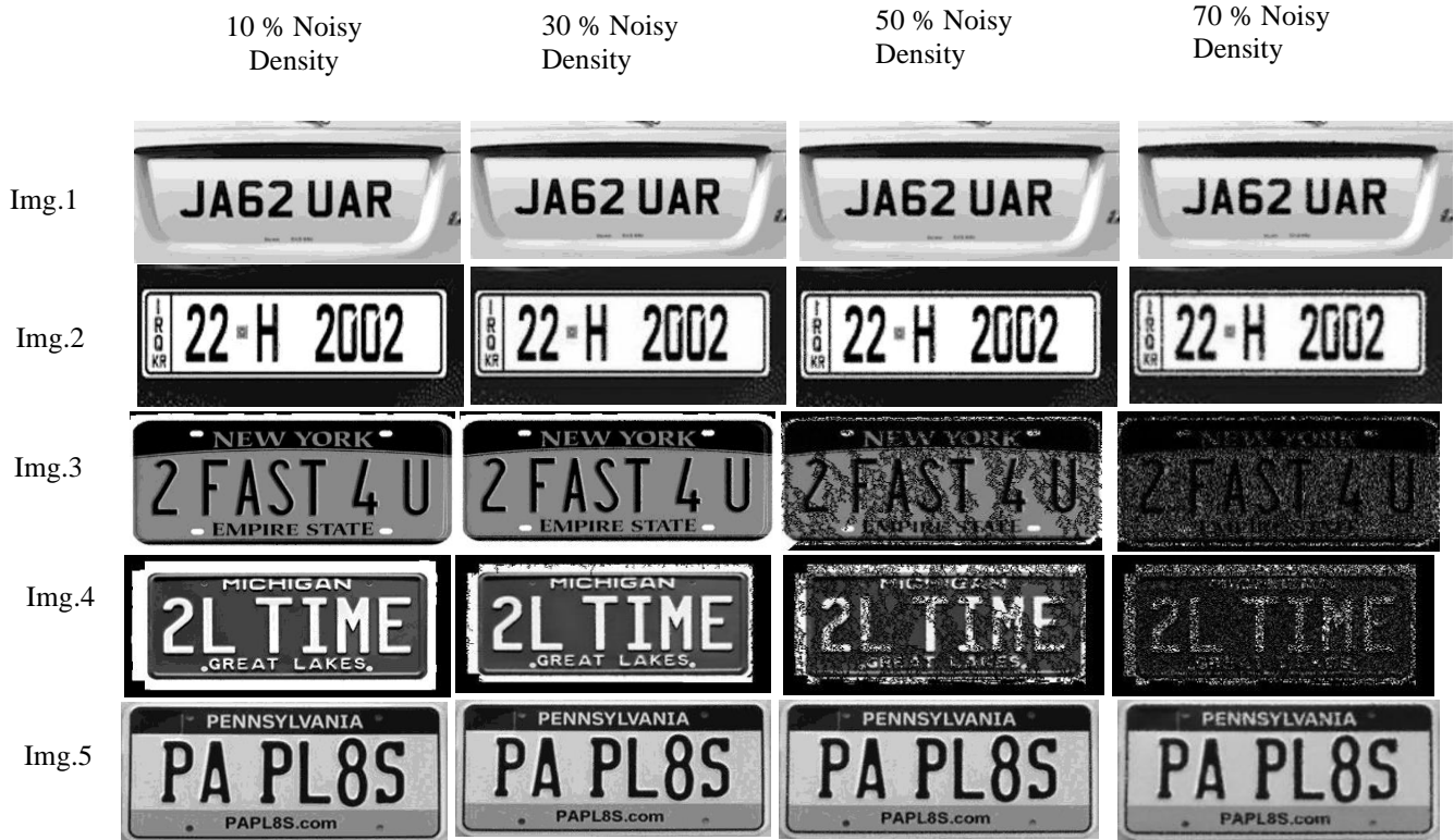
Fig. 5 Shows a set of images after removing different percentages of noise using the (NVBMF) filter
