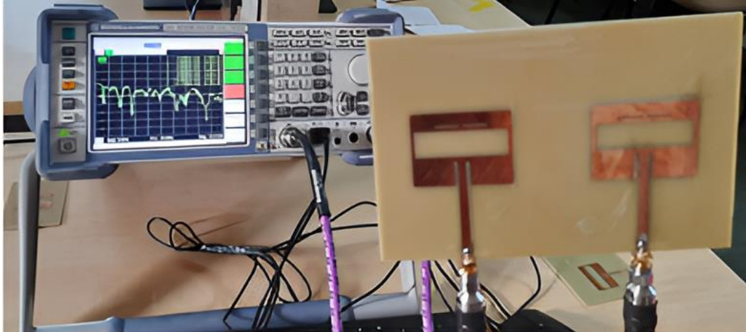
Fig. 19 VNA interfaced with the antenna
