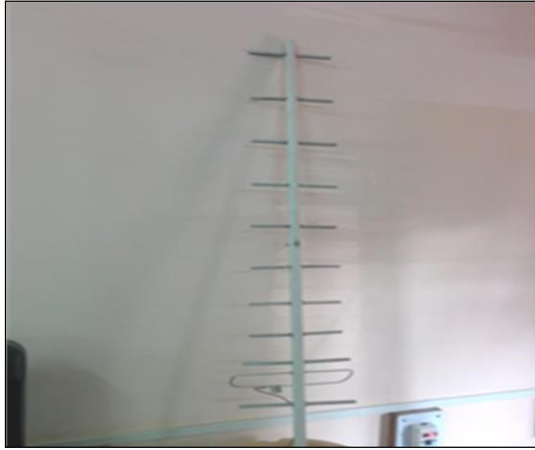
Fig. 6 Designed Yagi-Uda antenna for 2.4 GHz frequency
