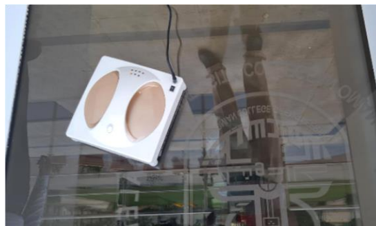
Fig. 4 Vertical surface cleaning test
