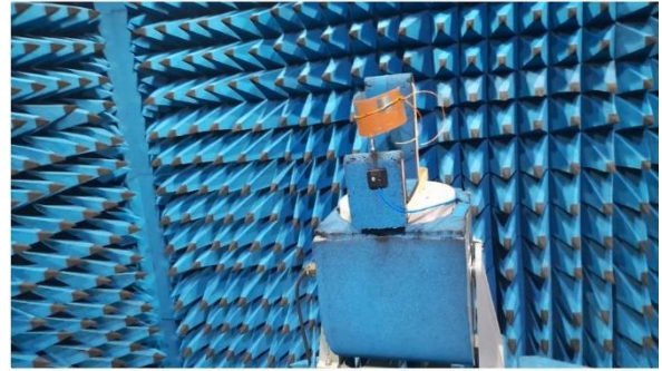
Fig. 7 Anechoic chamber mount
