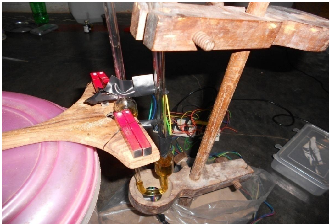
Pic. 1. Viscometer with Magnetic Field
