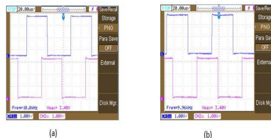
Fig 17: Switching pulses of the inverter (a) S_3 & S_4 (b) S_3 & S_5
