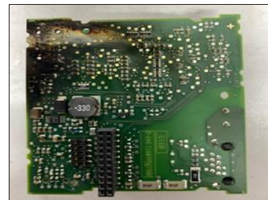
Fig. 13 PLC logo damaged by high voltage
