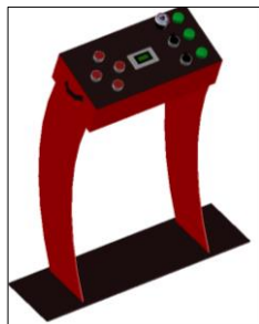
Fig. 24 Modified control panel design
