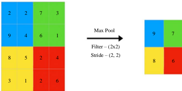
Fig. 11 Visualization of max pooling operation
